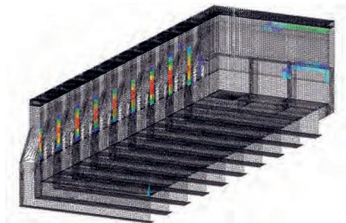
Fig. 3: Pressure applied on the 'empty shell' model potshell structure as boundary conditions
