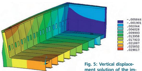
Fig. 5: Vertical displacement solution of the improved 'empty shell' model for the standard potshell design using the plastic mode (m)
