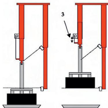
Fig. 5: Measuring the new anode height
