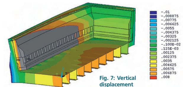
Fig. 7: Vertical displacement solution of the improved 'almost empty shell' model for the retrofitted potshell design using the plastic mode (m)
