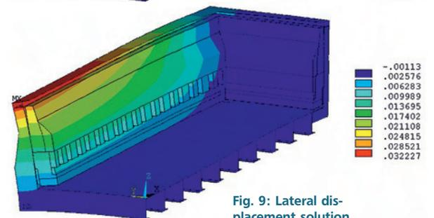
Fig. 9: Lateral displacement solution of the improved 'almost empty shell' using the plastic mode (m); top: standard potshell and lining design, bottom: retrofitted potshell and lining design
