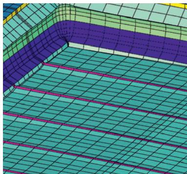
Fig. 8: Cathode panel erosion profile obtained using the full cathode panel erosion model
