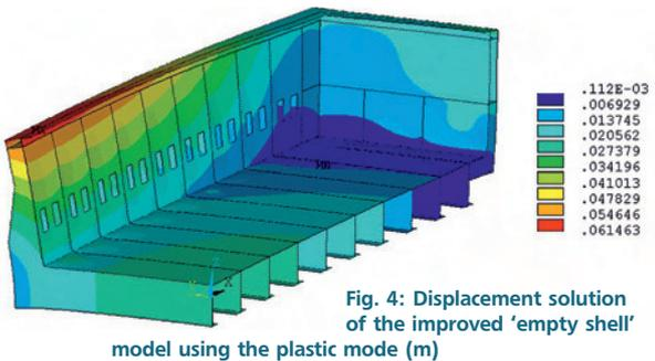
Fig. 4: Displacement solution of the improved 'empty shell' model using the plastic mode (m)
