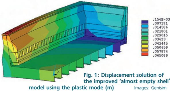
Fig. 1: Displacement solution of the improved 'almost empty shell' model using the plastic mode (m) Images: Genisim
