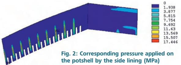
Fig. 2: Corresponding pressure applied on the potshell by the side lining (MPa)
