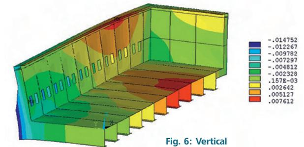
Fig. 6: Vertical displacement solution of the improved 'empty shell' model for the retrofitted potshell design using the plastic mode (m)
